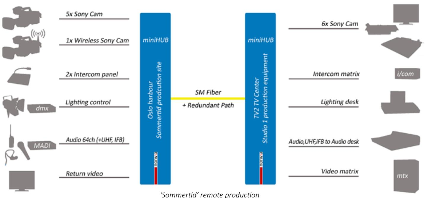
The Sony HDC-1500 cameras were operated by on location cameramen in coax mode. These 5 main cameras were connected to the miniHUB by 50m coax cable. Riedel keypanels were connected to the miniHUB and allowed for full control and connection back to the Studio. The UHF and IFB were also connected via the miniHUB. The Norwia miniHUB sent the video, audio and control signals to and from the studio over fiber.
